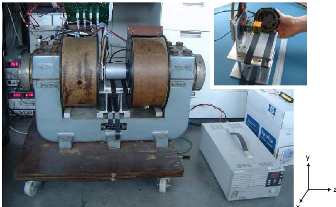
Figure 1: Magnet and MaPMT housing; corners: opened housing with the MaPMT and MaPMT coordinate system.
