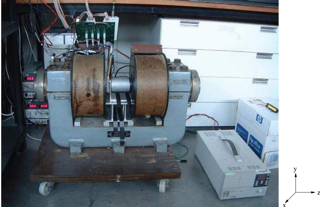
Figure 5.1: Magnet and MaPMT housing (See Appendix A.1 for an enlarged view of the opened housing with the MaPMT). The z-axis is defined as perpendicular to the photocathode of the tube, x is the horizontal transverse axis and y the vertical transverse axis.
