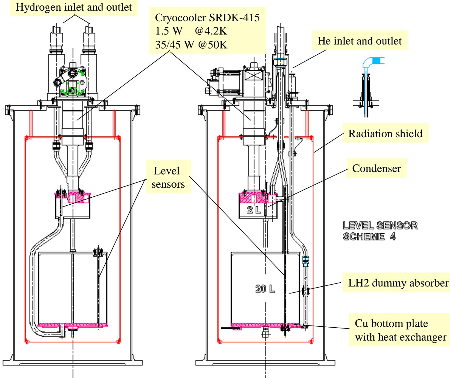
Dummy absorber and cryostat
