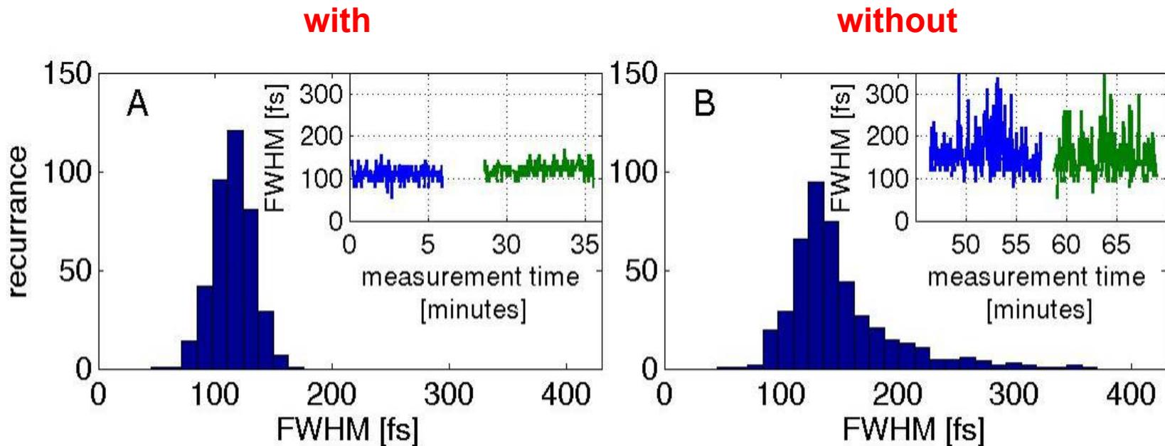
**Bunch profile FWHM at FLASH, with and without feedback system (CDR) running as measured by Dundee EO system**
