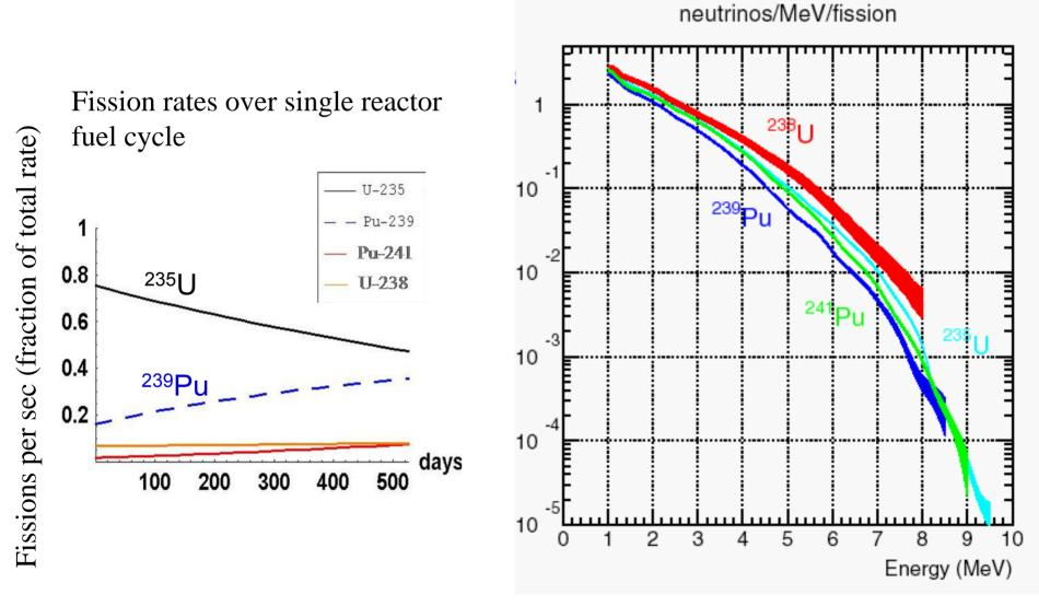
Plutonium breeding over fuel cycle(~250 kg over fuel cycle) changes antineutrino rate (by 5-10%) and energy spectrum
