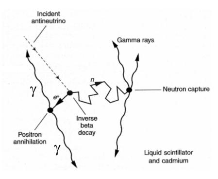
Signal was delayed coincidence between positron (2-5 MeV) and neutron capture on cadmium (2-7 MeV)
