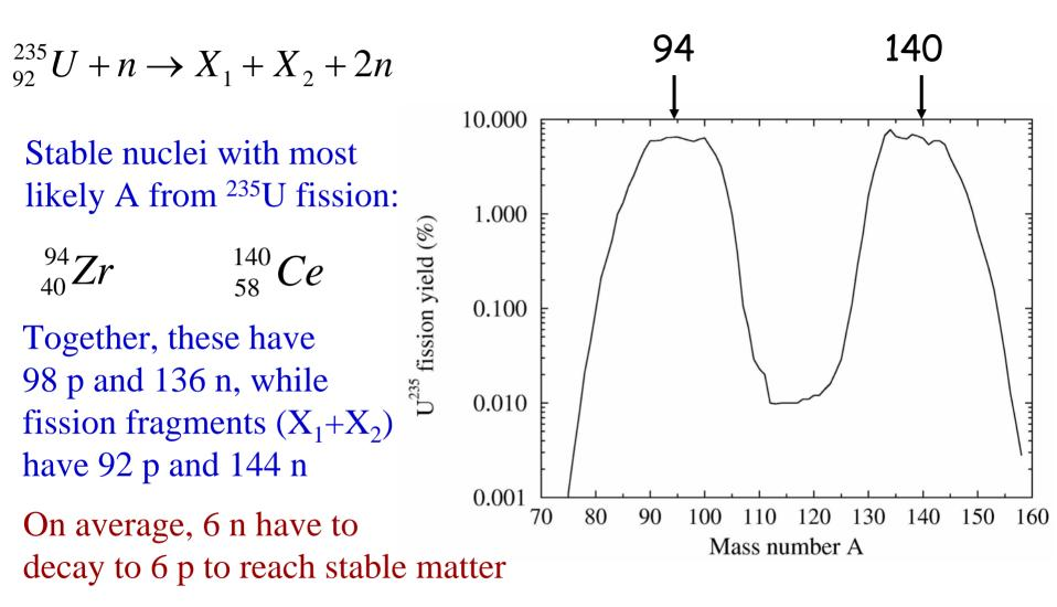
~ 200 MeV/fission and ~6  $\overline{v}_{e}$  / fission implies that 3GW<sub>th</sub> reactor produces ~ 6×10<sup>20</sup>  $\overline{v}_{e}$  / sec.
