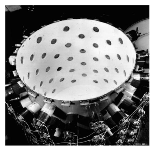
300 liters of liquid scintillator loaded with cadmium
