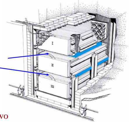
Inverse  $\beta$  decay would produce two signals in neighboring tanks (I,II or II,III):
