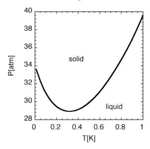
The figure shows the measured solid-liquid phase transition line for <sup>3</sup>He for temperatures from 0.010 K to 1 K. Pressure is measured in atmospheres.
