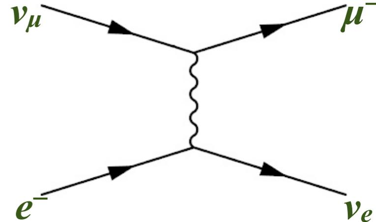
$$\mathcal{M} = \frac{g_W^2}{8} \bar{u}(\nu_e) \gamma^\mu (1 - \gamma^5) u(e^-) \frac{g_{\mu\nu}}{q^2 - m_W^2} u(\nu_\mu) \gamma^\nu (1 - \gamma^5) u(\mu)$$
