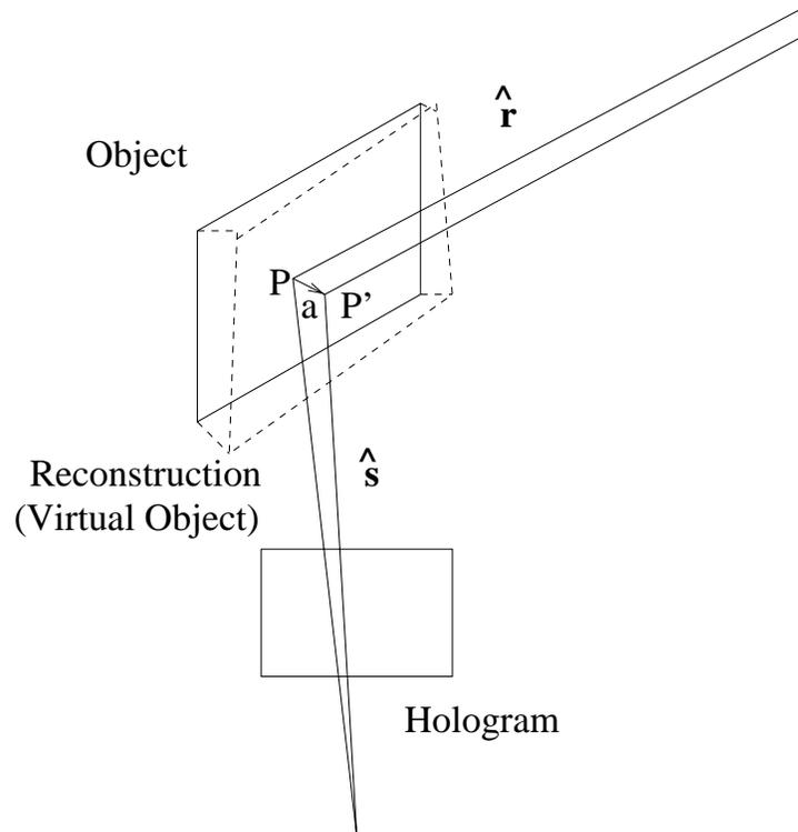
Point  $P$  on object moves to point  $P'$  on reconstruction (virtual object).
