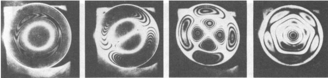
Vibrating guitar at (a) 185 Hz and (b) 285 Hz, from Molin & Stetson, Institute of Optical Research, Stockholm, (1971)
