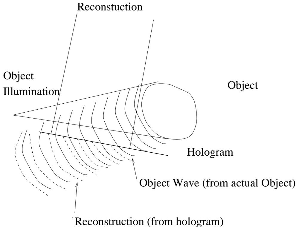
Interference between object and static reconstruction. Distort object, *Live Fringes*.
