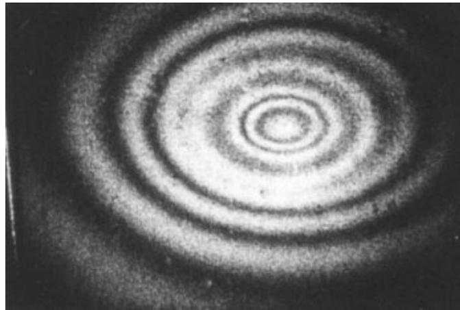
Live fringe image of convective mass transfer experiment of model AGR fuel-rod using swollen polymer technique.
