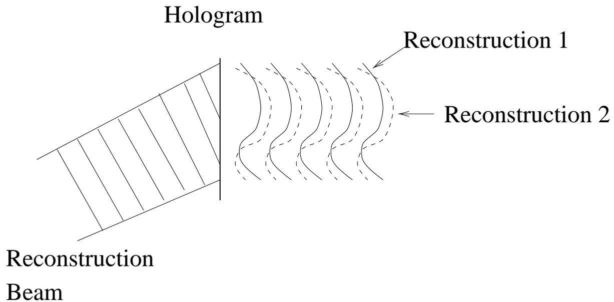
Two reconstructions will interfere and give fringes of constant OPD between the two reconstructions. (Measure difference from fringes).
