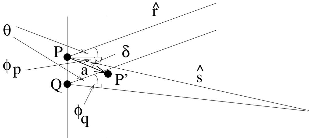
Where  $\theta$  is illumination direction,  $\phi_P$  and  $\phi_Q$  are viewing directions and  $\delta$  is angle of movement.
