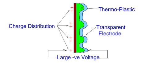
Apply Large voltage, plastic distorts under electrostatic attraction.
