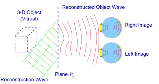
Reconstruct Amplitude Distribution in plane  $P_0$  we will still see the two images, and hence a 3-D virtual image of the original object.
