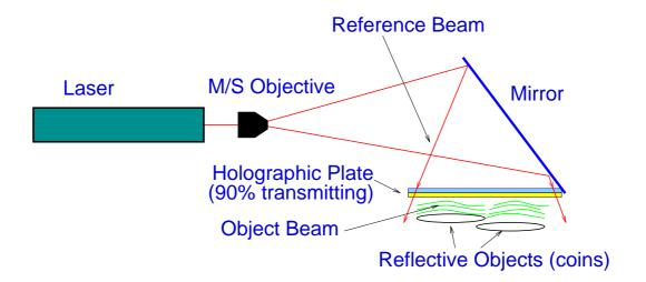
The reference and object illumination beam are combined and the object beam is reflected back from the objects.
