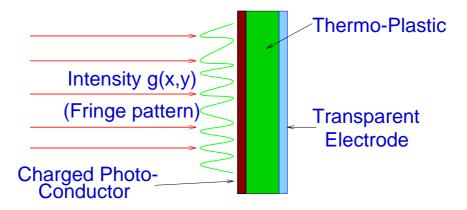
Expose to intensity g(x, y), surface change built-up proportional to the incident intensity.
