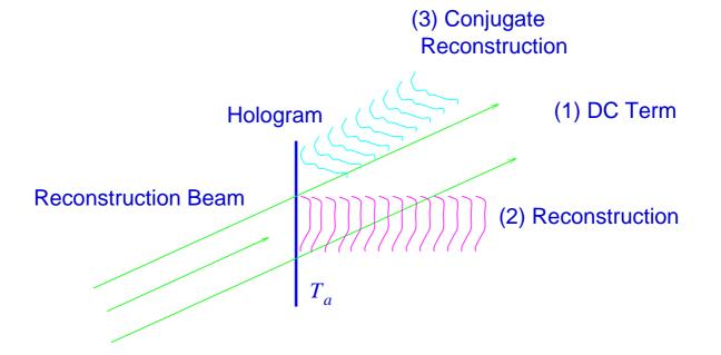
Three terms separated. Only want (2) which is full three dimensional reconstruction of object wave.
