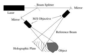
each "arm" contains one beamsplitter, one mirror and one microscope objective, so component efficiency losses are the same for each "arm". At the hologram we require that
