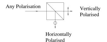
If we take the case of the input beam being *plane* polarised at angle  $\theta$  to the vertical then, from Malus' Law the *intensity* of the vertical and horizontally transmitted beams will be,
