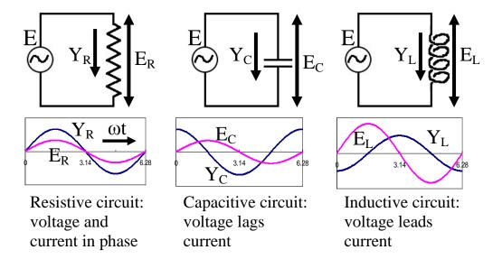
We have now completed the most **basic analysis of the LCR circuit** driven at an angular frequency,  $\omega$ , summarized below.
