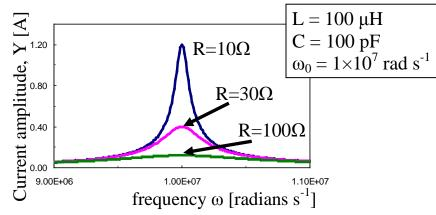
Next we can determine the width of the peak by finding the **full width at half maximum (FWHM)**, i.e. the width between the two points at which the current is half of its resonant value.
