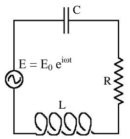
An **analogous mechanical setup** to this AC circuit is the following: a weight is suspended on a horizontal rail, on which it can move with friction. A spring is attached horizontally, which on the other side is forced by a sinoidal movement.
