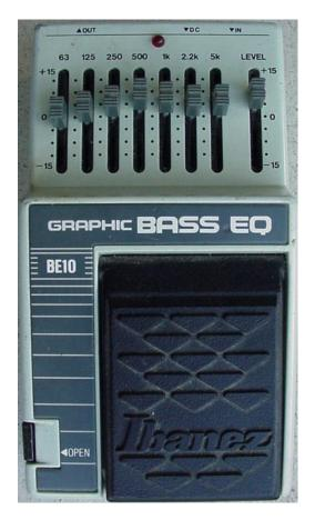
The oscillations of the strings of the guitar are picked up in a sensor and translated into **oscillations of a current** in a conductor. **Filter circuits** in the graphics equalizer, using the same principles we discussed in the last lecture, *split* the **frequency spectrum** into several bands, which in turn are routed through individually regulated amplifier stages, before they are *mixed* (merged) again into one signal.
