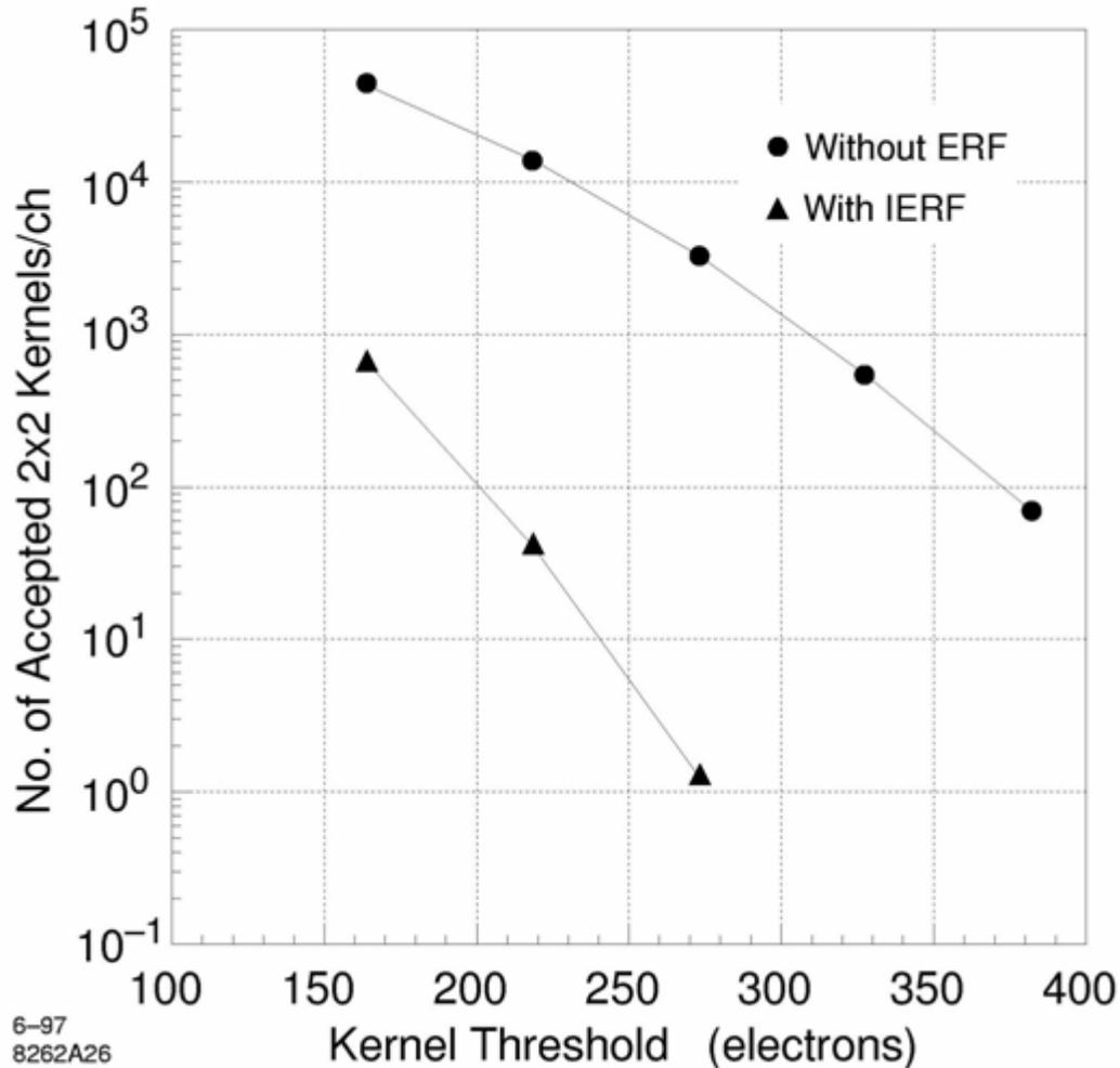
**Without ERF, rate of trigger pixels would have deluged the DAQ system**
