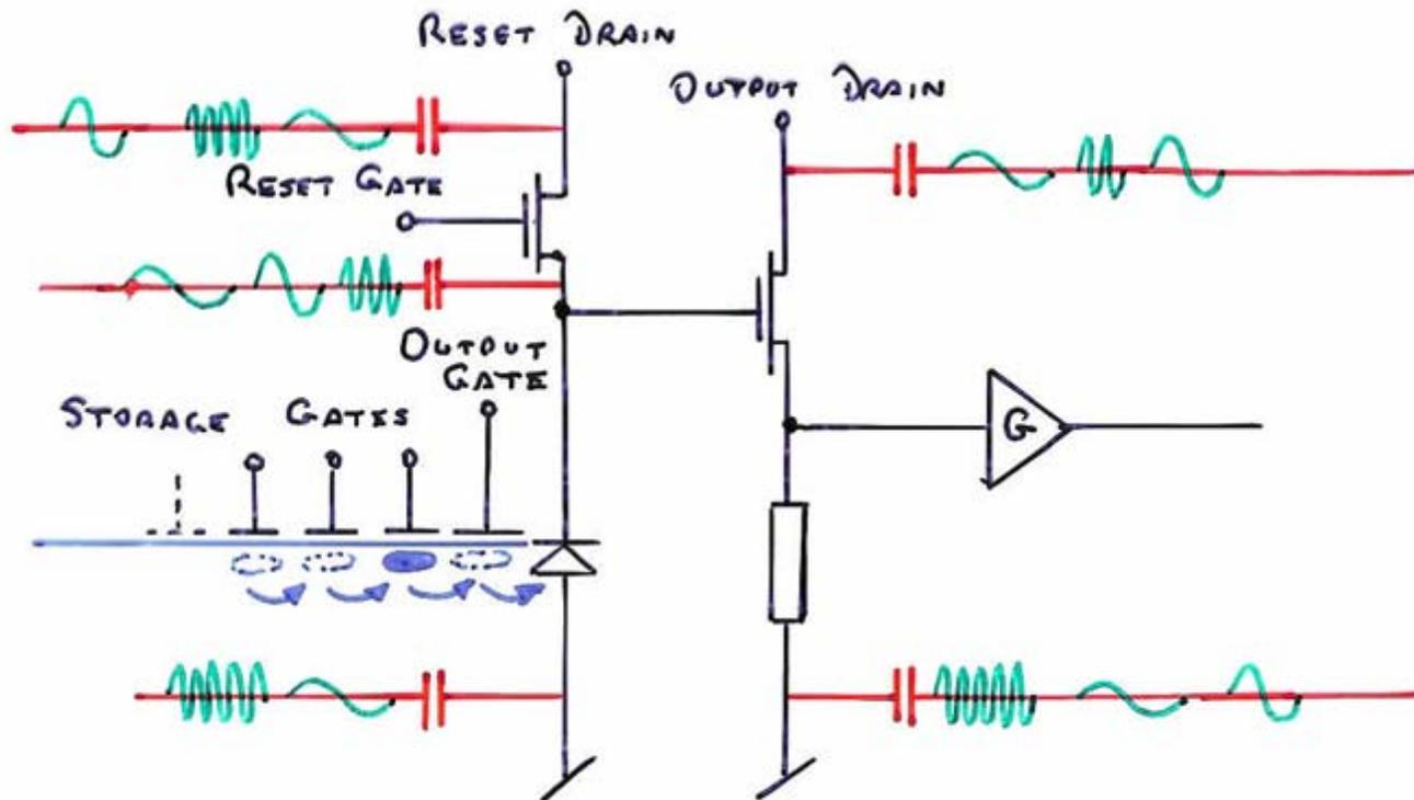
From SLD experience, signal charges stored in buried channel are virtually immune to disturbance by pickup. They were transferred in turn to the output node and sensed as voltages between bunches, when the RF had completely died away
