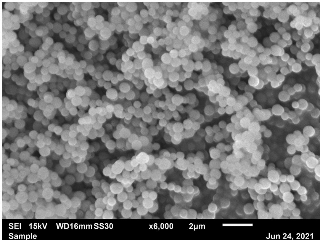
*Figure 1: Scanning Electron Microscopy (SEM) image of the batch of silica particles used for bijel fabrication. See “Experimental Section” in main text for further details.*
