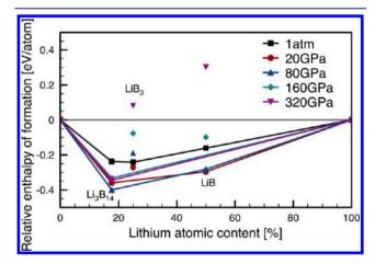
**Figure 3.** Ground-state enthalpies of formation for experimentally known  $\text{Li}_x B_y$  phases, shown as a function of Li atomic content, and for various pressures. Enthalpies are relative to the crystalline elements.
