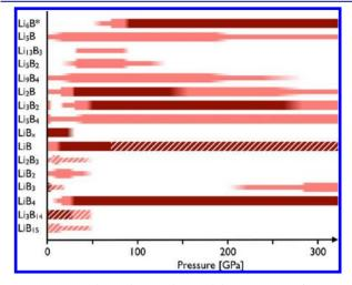
**Figure 21.** Ground-state binary phase stability ranges as a function of pressure. Dark red (light red, thin light red) lines denote, respectively, stable structures, structures within 50 meV/atom of stability, and structures within 100 meV/atom of stability. LiB<sub>x</sub> refers to compositions with  $0.8 \le x \le 1.0$ . Structures that we find nonmetallic are indicated by striped patterns. \*The Li<sub>6</sub>B structure is the one kindly given to us by Prof. Ma.
