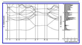
**Figure 15.** Electronic band structure (left) and DOS (right) of the ground-state *Cmcm* phase of  $Li_2B$ , at P = 1 atm. Dashed line in the DOS plot indicates projection onto boron atoms within the atomic pseudo-cutoff radius. Note the large density of states right at the Fermi level.
