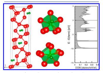
**Figure 16.** Left: ground-state  $\text{Li}_9\text{B}_4$  phase, in the  $\text{Li}_9\text{A}_4$  structure. Optimized structure at P = 1 atm is shown, with B–B separations  $\leq 2$  Å and Li–Li separations  $\leq 3.2$  Å drawn as connected. Middle: the coordination polyhedra of the boron atoms, with separations  $\leq 2.7$  Å drawn as connected. Right: the electronic DOS at P = 1 atm, exhibiting a rather large DOS at the Fermi level.
