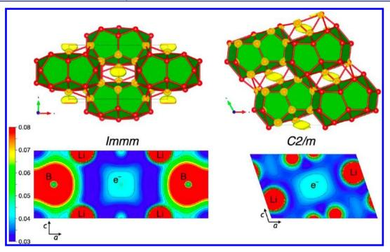
**Figure 20.** Top: *Immm* (left) and C2/m (right) structures of Li<sub>5</sub>B at P = 160 GPa, both with ELF isosurfaces (ELF = 0.85). Bottom: corresponding electronic charge density profiles, both for cuts along the [010] direction. Units are  $e/Å^3$ .
