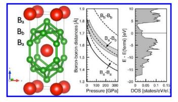
**Figure 13.** Ground-state LiB<sub>4</sub> phase in the BaAl<sub>4</sub> structure type. Left: optimized crystal structure at P = 80 GPa. Middle: B–B separations in LiB<sub>4</sub> (dashed lines) compared to B–B separations in pure boron (solid lines, see also Figure 4). Right: DOS at P = 80 GPa (where  $V/V_0 = 0.78$ ).
