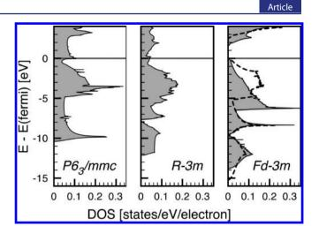
**Figure 10.** Electronic DOS per valence electron of LiB structures. From left to right: experimental structure at P = 1 atm; the proposed sandwich structure at P = 40 GPa ( $V/V_0 = 0.62$ ); and the NaTI structure type at P = 80 GPa ( $V/V_0 = 0.71$ ). Energies are relative to the respective Fermi levels or valence band maximum (VBM). Dashed line in the NaTI structure DOS plot is the DOS for pure diamond, taken at the lattice constant of LiB at P = 80 GPa.
