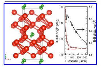
**Figure 14.** Left: ground-state  $Li_2B$  phase at P = 1 atm in the  $ZrSi_2$  structure, also found in  $Li_2Ga$ . Right: evolution of (i) the shortest B–B distance, and (ii) the B–B–B angle within the kinked chains with pressure.
