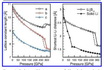
**Figure 7.** Evolution of lattice constants (left) and shortest Li–Li distances (right) in the experimental structure of  $\text{Li}_3\text{B}_{14}$  under pressure (the Li–Li separations compared to the distances in solid lithium). Solid (dashed) lines are results from ground-state calculations with increasing (decreasing) pressure. The discontinuities are associated with phase transitions.
