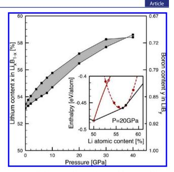
**Figure 12.** Shaded area is the ground-state stability range of borondepleted chain structures based on the experimental LiB structure, as a function of pressure. The inset illustrates how the data points in the main figure are obtained: by finding the correct points of the enthalpy parabola, whose tangents are parts of the convex hull of stability.
