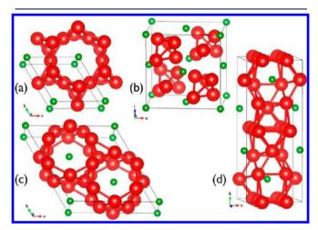
Figure 17. Common ground-state  $AB_5$  structures in intermetallic compounds: (a) P6/mmm (CaCu<sub>5</sub>); (b)  $F\overline{4}3m$  (AuBe<sub>5</sub>); (c) P6/mmm (YNi<sub>2</sub>Al<sub>3</sub>); and (d) *Cmcm* (BaZn<sub>5</sub>). Li atoms are red, B atoms are green.
