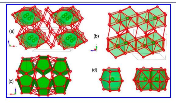
**Figure 19.** (a) Ground-state  $P2_1/m$  structure for  $Li_5B$  and (b)  $P\overline{1}$  structure, both at P = 60 GPa. (c) *Cmma* structure at P = 160 GPa. (d) Boron atom and dimer cages found in the high-pressure phases of  $Li_5B$ .
