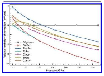
Figure 9. Relative ground-state enthalpies of formation of various LiB phases in the ground state.
