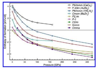
Figure 18. Relative ground-state enthalpies of formation per  $Li_{s}B$  unit, normalized to elemental B and Li crystals.
