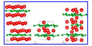
**Figure 11.** Ground-state structures of  $Li_5B_4$  and  $Li_3B_2$ : left,  $Li_5B_4$  at P = 1 atm; middle,  $Li_5B_4$  at P = 80 GPa; right,  $Li_3B_2$  at P = 80 GPa (all drawn on the same length scale).
