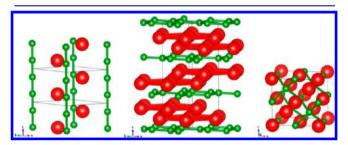
**Figure 8.** Sequence of crystal structures for 1:1 LiB. From left to right: the experimental structure at P = 1 atm, the proposed ground-state sandwich layer structure at P = 40 GPa, and the NaTl Zintl phase at P = 80 GPa. All structures are drawn to the same scale.
