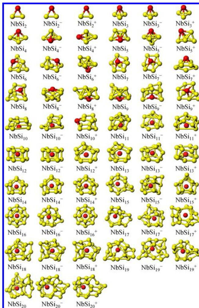
**Figure 2.** Lowest energy structures of  $\text{NbSi}_n^Q$  ( $n = 2–20$ ;  $Q = 0, \pm 1$ ) clusters. The red (yellow) spheres represent the Nb (Si) atoms.
