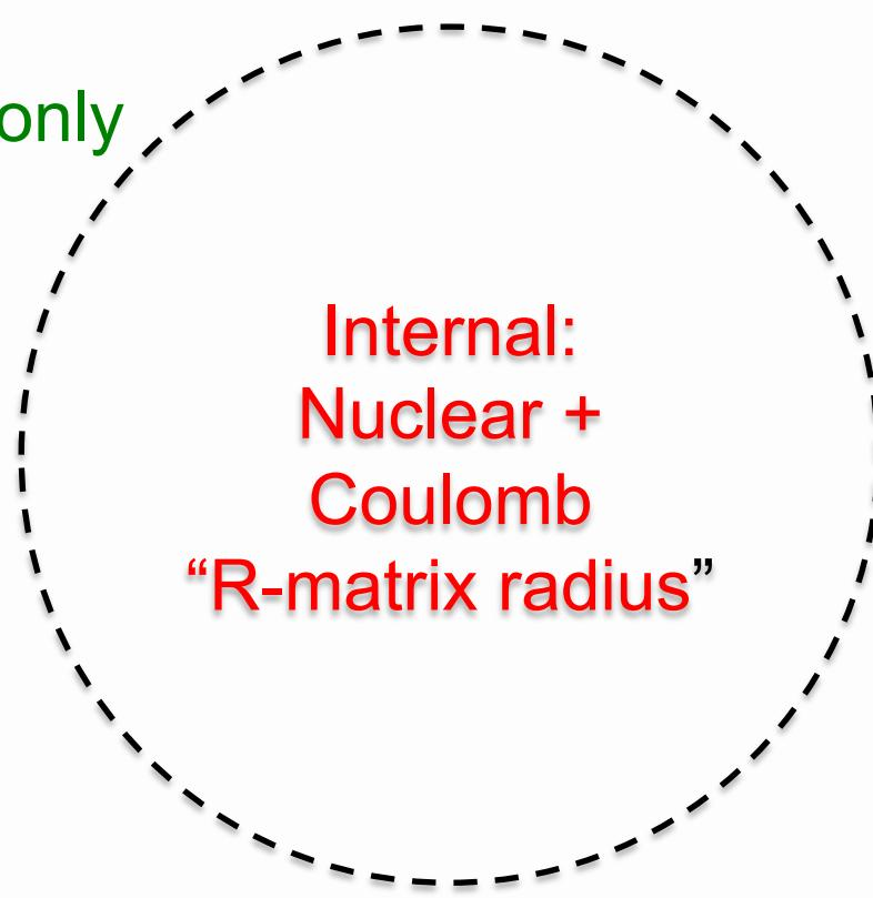
A diagram illustrating the R-matrix formalism. A dashed circle represents the system's boundary. The interior of the circle is labeled "Internal: Nuclear + Coulomb" and "R-matrix radius" in red text. The exterior of the circle is labeled "External: Coulomb only" in green text.
