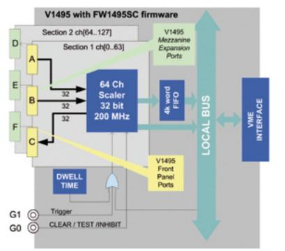
The counters can be also read out "On the fly" real time via VME. A programmable General Input signal (NIM /TTL) can be programmed as CLEAR, TEST or VETO (in common for all channels).
