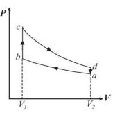
The 'Otto cycle' is an idealisation of the internal combustion engine. Which segments represent fuel compression, burning, and exhaust?
