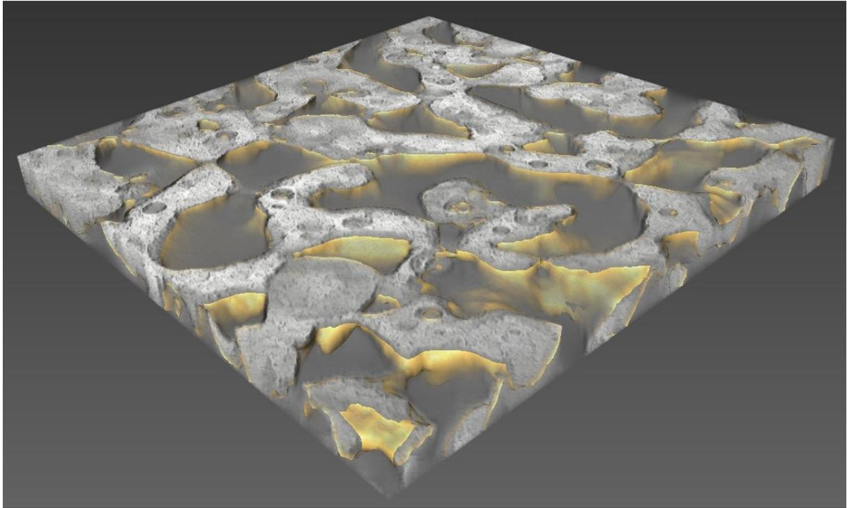
Supplementary Figure 3: A 3D volume rendering of a microparticle stabilized bijel (greyscale) with the calculated isosurface superimposed (yellow). The isosurface clearly follows the pattern of the raw data, meaning that the curvature analysis performed on the isosurface can be said to represent the curvature values of the raw data, i.e. the bijel.
