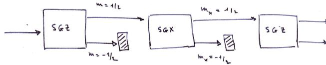
Figure 14.1: A beam of atoms, each with  $j = \frac{1}{2}$ , travelling along the  $y$ -axis passes through a sequence of Stern-Gerlach magnets whose mean fields are oriented along either the  $z$ -direction (SGZ) or the  $x$ -direction (SGX). The shaded boxes represent absorbers.
