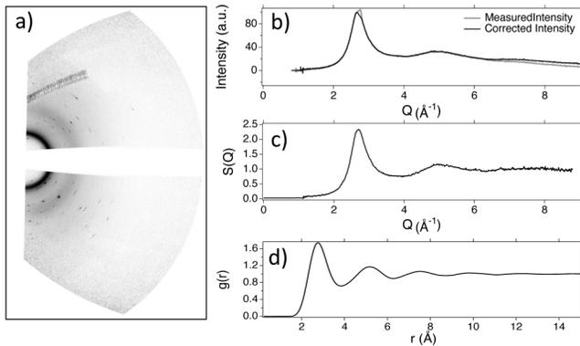
**FIG. 7.** Structural analysis of liquid Sn—shot 831. (a) 2D diffraction image warped into a geometric view such that diffraction rings are concentric circles. (b) 1D integrated line out from uncorrected and corrected data. (c) Optimized  $S(Q)$  profile. (d) Optimized  $g(r)$  profile.
