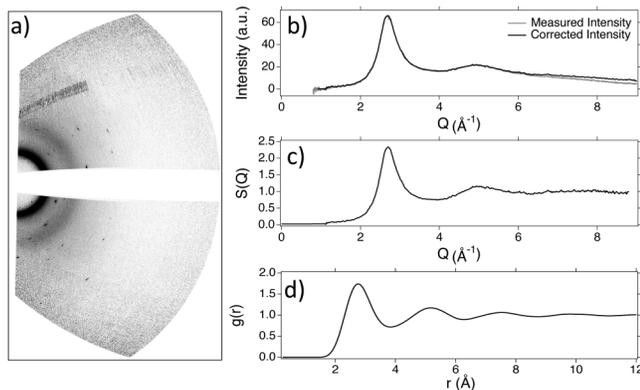
**FIG. 5.** Structural analysis of liquid Sn—shot 826. (a) 2D diffraction image warped into a geometric view such that diffraction rings are concentric circles. (b) 1D integrated line out from uncorrected and corrected data. (c) Optimized  $S(Q)$  profile. (d) Optimized  $g(r)$  profile.
