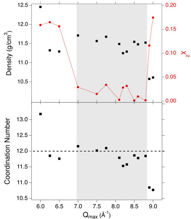
**FIG. 8.** Effect of  $Q_{\max}$  on optimization—shot 831. Density and  $\chi^2$  (top) and coordination number (bottom) was determined as a function of  $Q_{\max}$ . The figure of merit  $\chi^2$  (red) is minimized between 7.0 and 8.8  $\text{\AA}^{-1}$ .
