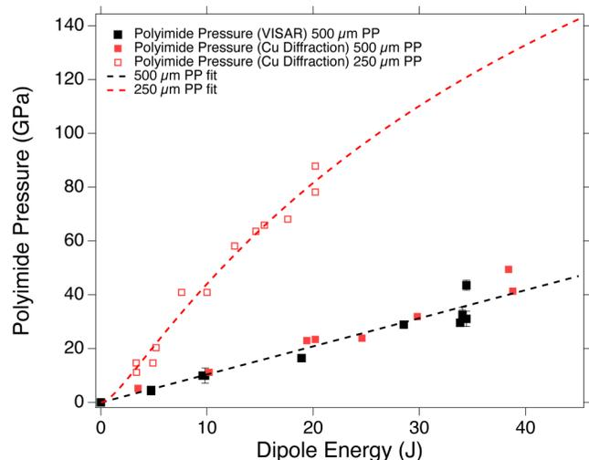
FIG. 3. Polyimide pressure as a function of laser energy for 500 and  $250\ \mu\text{m}$  phase plates (PPs). This relation was determined by two independent methods: using impedance matching from VISAR traces from polyimide-LiF targets (black); using impedance matching from Cu diffraction data from polyimide-Cu targets (red).
