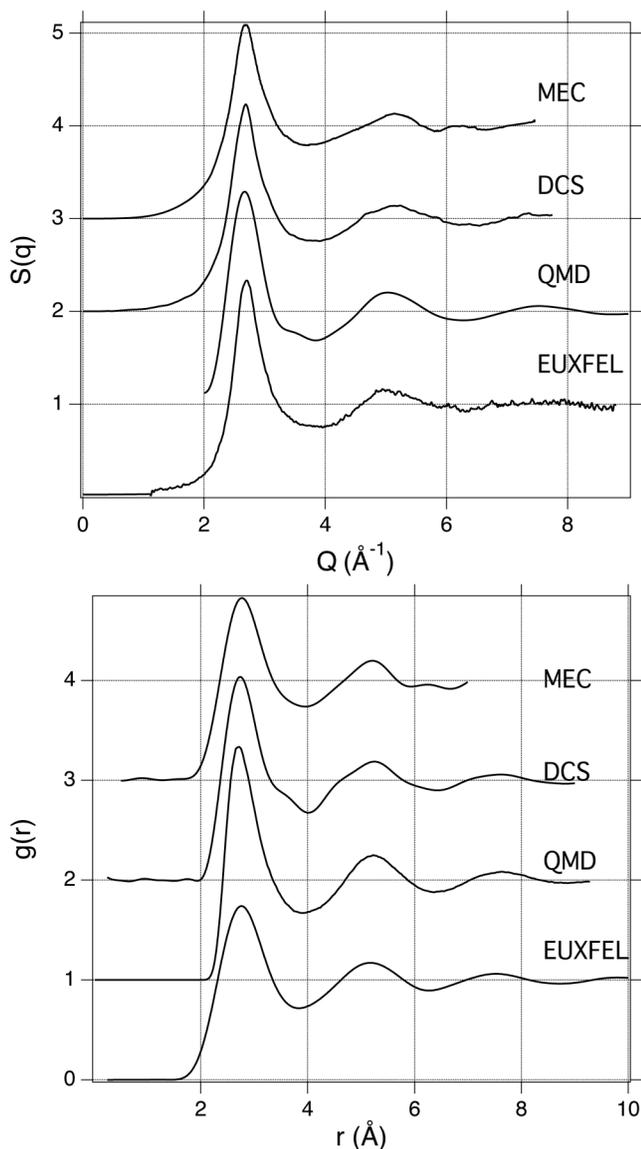
**FIG. 9.** Comparison with other facilities and simulation.  $S(Q)$  (a) and  $g(r)$  (b) data from this work compares well with similar measurements performed at DCS and MEC as well as the results of QMD simulations performed at similar conditions. The accuracy of the measurements at MEC and DCS were hindered by experimental constraints (see text).
