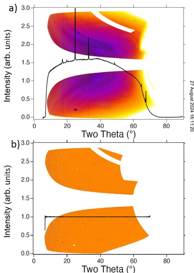
**FIG. 4.** Flat-fielding the Varex detectors. YAG crystal was illuminated with EuXFEL beam to induce fluorescence emission. (a) Uncorrected image from Varex detectors with accompanying line out. (b) Corrected image with parasitic Bragg reflections masked out.<sup>24</sup>
