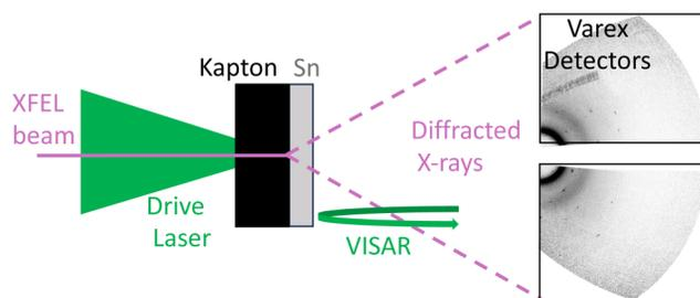
**FIG. 1.** Experimental setup. The target design consists of a 50  $\mu\text{m}$  thick polyimide ablator bonded to a 20  $\mu\text{m}$  thick Sn foil with a  $\sim 1$   $\mu\text{m}$  glue layer. Diffraction data from laser shock compressed Sn at an estimated pressure of 85 (5) GPa are shown. The 2D diffraction images were generated using the HEXRD diffraction software package.<sup>13</sup>
