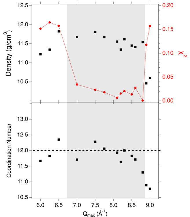
**FIG. 6.** Effect of  $Q_{max}$  on optimization—shot 826. Density and  $\chi^2$  (top) and coordination number (bottom) as determined as a function of  $Q_{max}$ . The figure of merit  $\chi^2$  (red) is minimized between 7.0 and 8.8 Å<sup>-1</sup>.
