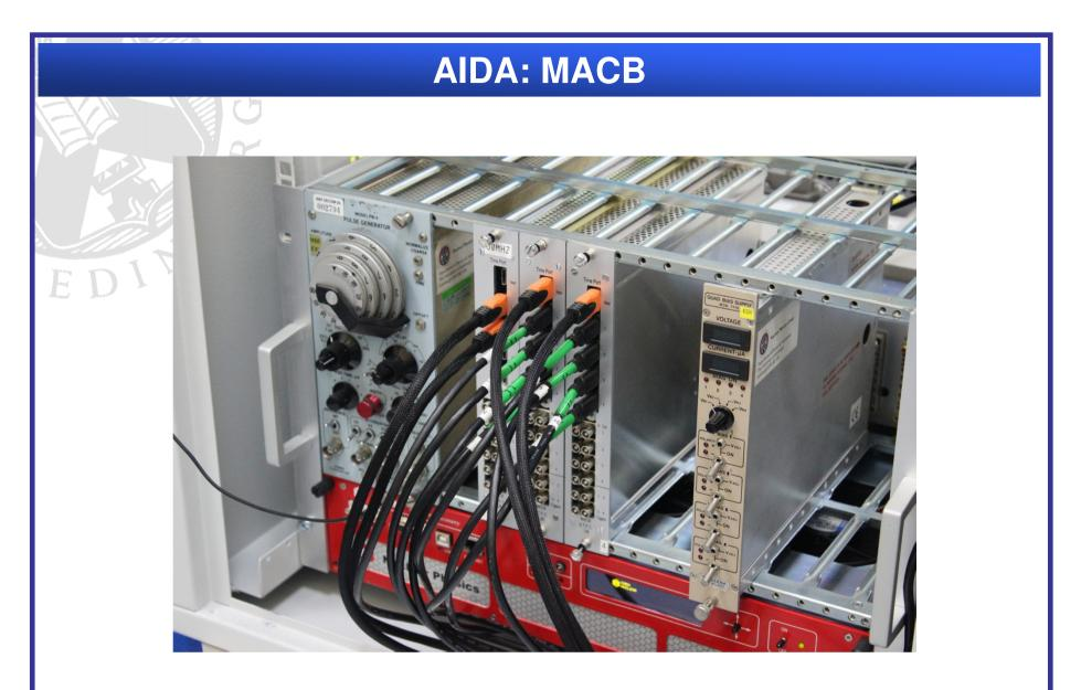
Timestamping hardware with HDMI cabling to AIDA FEE modules
