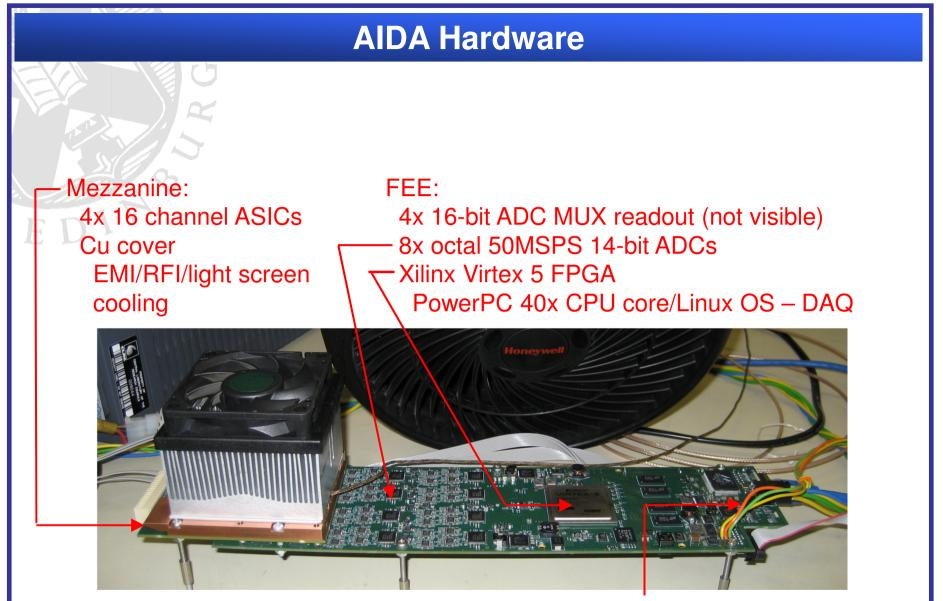
FEE width: 8cm Prototype – air cooling Production – recirculating coolant Gbit ethernet, clock, JTAG ports Power
