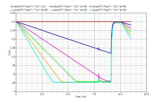
Constant current input: Full-scale 1µA for 10µs 0 to 5µA by 1µA steps Clamp enabled
