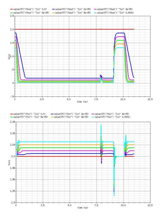
Constant current input: Full-scale 1µA for 10µs 0 to 100µA by 20µA steps Clamp enabled
