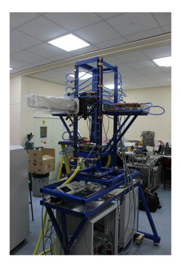
*'All up' tests in T4 laboratory STFC Daresbury Laboratory Note Julabo Recirculating Chiller to side of assembly*
