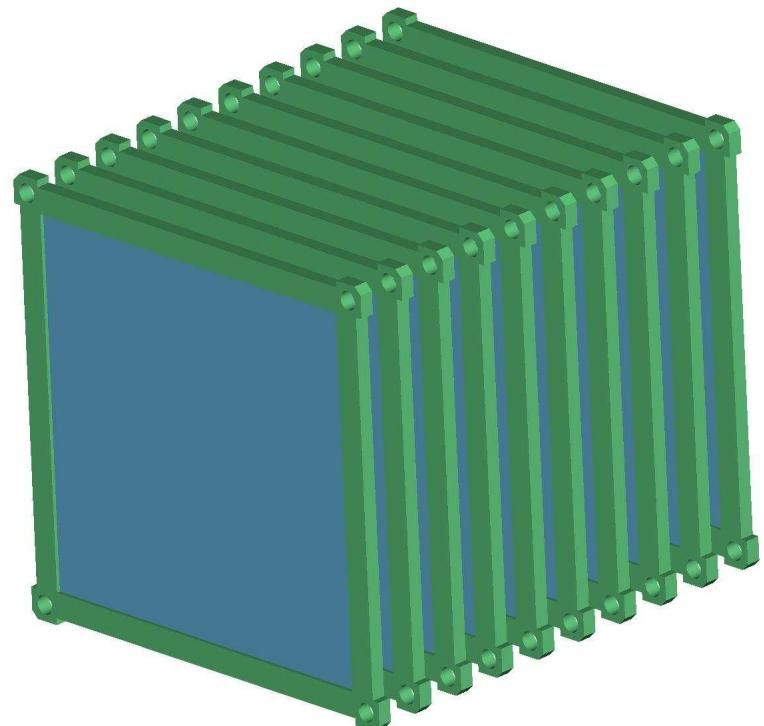
Si thickness = 1 mm, strip pitch = 625  $\mu\text{m}$ , >5000 channels
