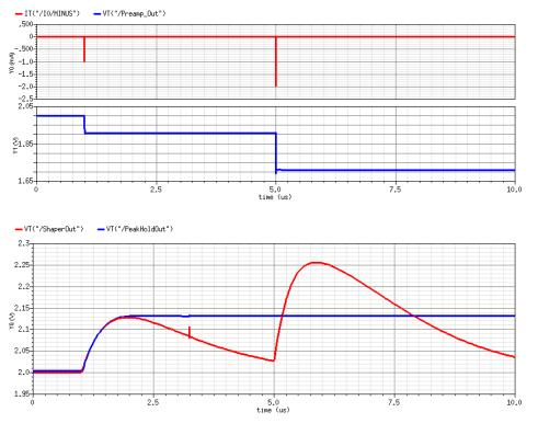
Detector current (1pC, 2pC) Pre-amp output (Cf=10pF)
