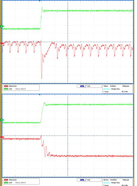
Input: 15ns 4.4V step on 10pF Output: Variable step with oscillation
