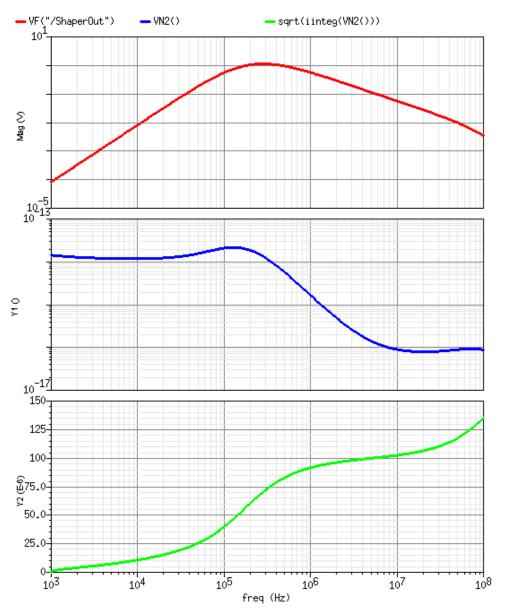
Analysis based on small-signal AC model : noise sources multiplied by AC transfer function to output.
