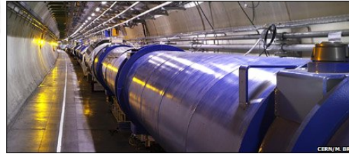
Superconducting magnets are cooled down using liquid helium
