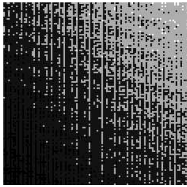
Figure 1: Image of an almost evenly illuminated blank card using a CCD camera showing fixed pattern noise.
