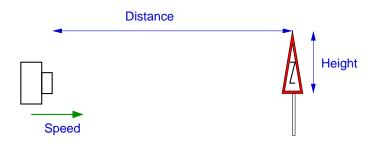
As car approached road we want to detect edges from one particular plane, so if the sign is in this plane, we will then detect the sign of the right size and ignore all other edge points in the image.
