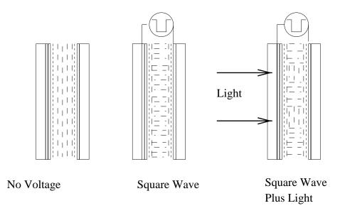
No applied voltage the molecules are "aligned" by the surface groves.
