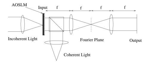
where the "outside-world" is imaged onto the OASLM, this image is then processor by the "4-f" system. (Laboratory project).
