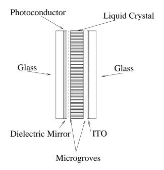
with the LC in a thin cell with surface groves that align the molecules.
