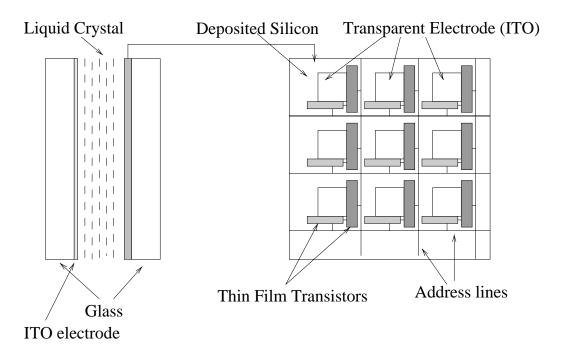
Address the "pixels" to change the local electric field across the liquid layer and hence switch pixels on or off. Add "grey-level" by altering the time each pixel is on for and colour by placing an array of colour filters on top of the display to group pixels in threes.
