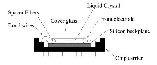
the silicon backplane is then essentially a "memory chip" with reflective mirrors.
