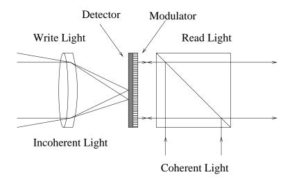
The "incoherent" light is detected (as intensity), by a photo-detector (as an electrical change distribution).
