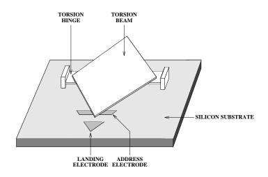
where each mirror is controlled by electrostatic force. So when a mirror is "tilted" it deflects the light "out of the system".
