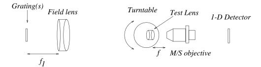
The one-dimensional detector would typically be a photo-diode array with a typical detector spacing of  $\approx 25\mu\text{m}$ , which is about 40 per mm, so to get an accurate measure of a 80 lines/mm pattern it must be multiplied by *at least*  $\times 4$ ,  $\times 10$  would be better.
