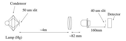
with the source slit illuminated by a incoherent source (for example a mercury lamp), and the 40µm slit translated infront of a large area photodetector to record the linescan.
