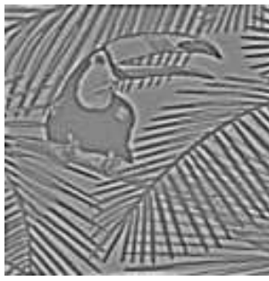
Figure 8: Laplacian of Gaussian filter applied to an image.
