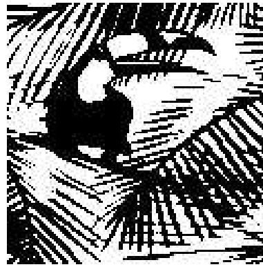
Figure 4: Example of binary threshold, giving a binary output image with pixels set to 0 and 255 only.
